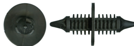
FA 4182 $0.90 Grille & Shroud Retainer Hole size 5/16 washer 3/4 O/L 1-7/16 1991 up GM Olds Bravada/Blazer
